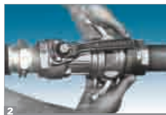
2 Cam arms lock coupler and adaptor together
